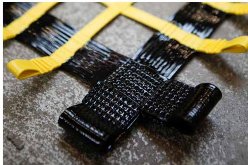
Roblon composite net used as safety protection on drilling rigs
